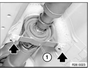
Grip propeller shaft and release nuts.
